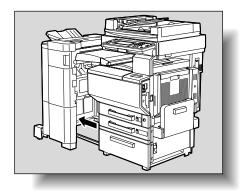
2 Open the horizontal transport unit cover, and then remove any misfed paper.
